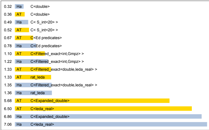
Fig. 10. Running times for different kernels supporting exact computation and for C<double> for 1000 points in a disk with algorithms Handley (Ha) and Akl-Toussaint (AT).
